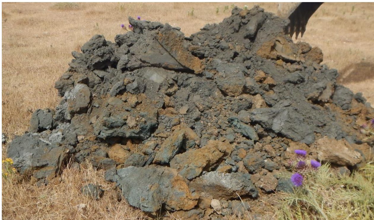
Fig. 4-4 Area 3 – Trincea esplorativa TP9 (1,5-2,0 m). Argille AT e ATa
